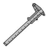
**Vernier caliper** – used for measuring thicknesses and diameters very precisely, in some cases to an accuracy of 10 micrometres, or 0.01 mm.
