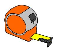
When you look closely at the end of a normal retractable tape, you'll notice that the steel hook is secured with rivets, with a bit of play in the holes allowing it to move back and forth. The amount of movement allowed is the same as the thickness of the hook.
