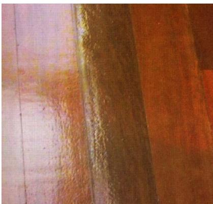
Orange peel has a slightly rough, orangey appearance. It happens when the solvent evaporates before the solids in the solution have time to spread evenly over the surface.
