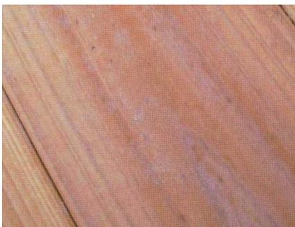
Crystallisation appears as a white discolouration in the coating. It can occur in cold weather with water-based polyurethanes and fast-dry sealers as they dry.
